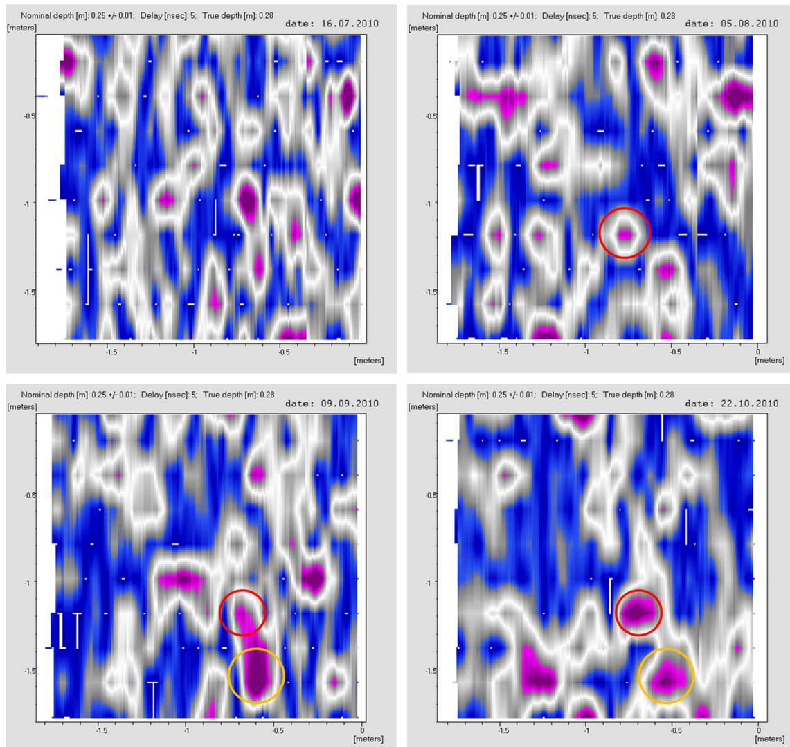
**Fig. 3** Radargrams from the permanent surface 1 at 28 cm depth; the truffle signals are the red/violet spots. The signal of a truffle harvested matures on 27 November is circled in red; the yellow circle indicates the signal of the second truffle harvested not completely mature during the same digging
